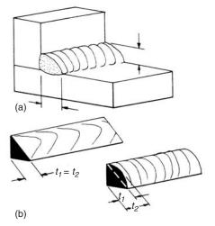
$5.6~{\rm Throat}$  thickness in a fillet weld: (a) fillet weld; (b) mitre and convex fillet weld.
