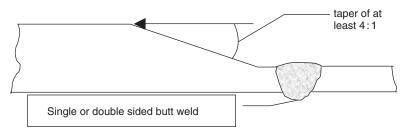
5.9 Suggested design for the joining of dissimilar thickness plates.
