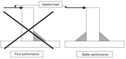
5.15 Redesign of side loaded fillet welds for improved performance.
