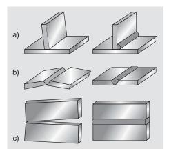
5.22 Presetting of components before welding. Courtesy of TWI Ltd.
