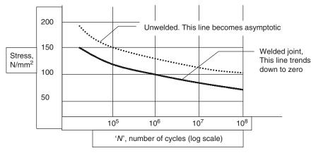
5.25 Stress/no. of cycles curve for alloy 5083.
