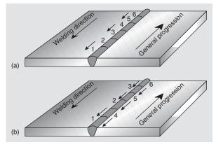
5.21 Backstep welding. Courtesy of TWI Ltd.
