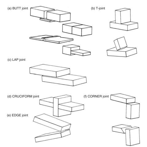
5.4 Joint types developed from the butt, fillet and edge weld.
