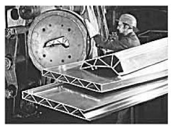
5.11 Typical self-jigging extrusions. Courtesy of ALCAN.
