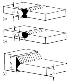
*5.5* Throat thickness in a butt weld: (a) full pen butt weld; (b) partial pen butt weld; (c) T-butt weld.
