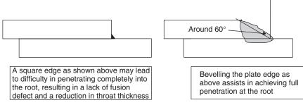
5.16 Bevelling the plate edge in a lap joint to improve penetration.
