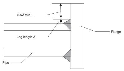
5.14 Recommended distance of weld toe from the flange edge.
