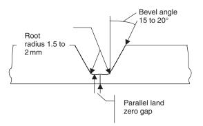
For AC-TIG welding the land should be 4.5 mm min, for DC -ve TIG and MIG the land should be 2 mm min
