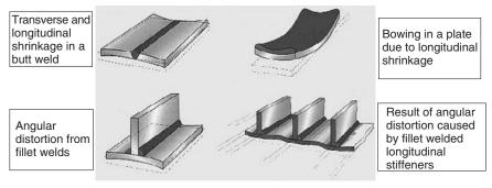
5.18 Longitudinal, transverse and angular distortion. Courtesy of TWI Ltd.
